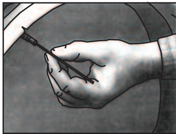
Run a wire through the valve stem to ensure tire is completely deflated.
